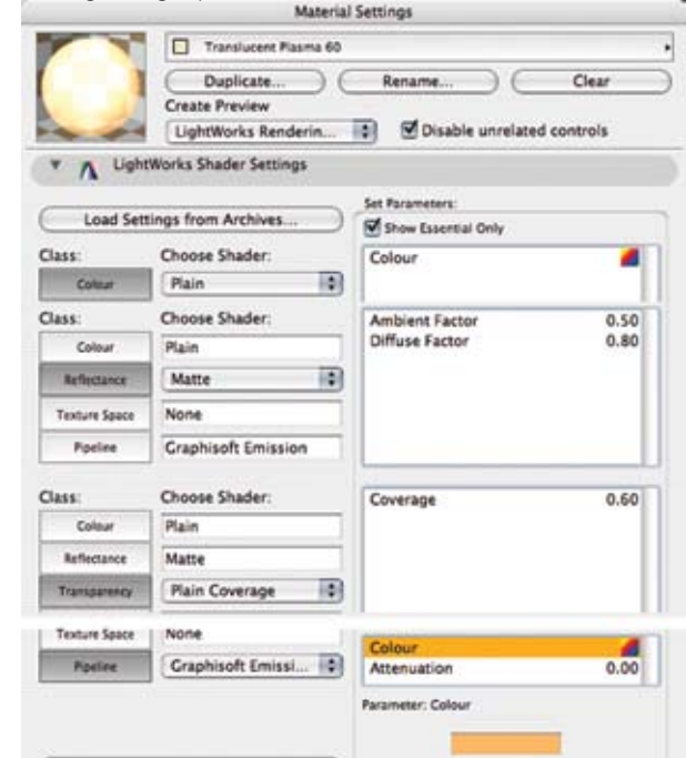
Emission Attenuation = 0 results in lack of modeling, just like a glowing object should.
